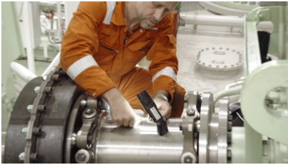
Installation of power measurement system on a thruster drive shaft
